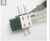
Trim the excess wire flush with the cover. It's recommended the tip of wires is not more than 0.2mm.
