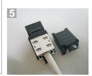
Use KJ-TLM series to terminate and cut 4-pairs of wires simultaneously finishing installations. Snap the jack's cover back on, over the wires.
