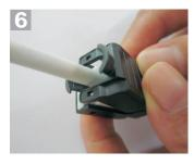
Place the wing cap over the terminated wires for secure connection .
