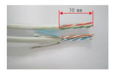
Strip approximately 30mm of the cable jacket, cut off the plastic cross, and separate the wire into 4 pairs.
