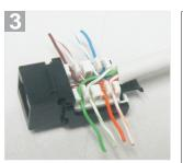
Terminate one pair at a time starting from rear of connector. Install each pair after replacement will repvent crushing theinside pairs with the punchdown tool.
