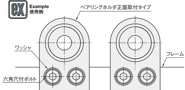
BEARING WITH HOUSINGS - FRONT INSTALLATION SHOULDER REST TYPE-
